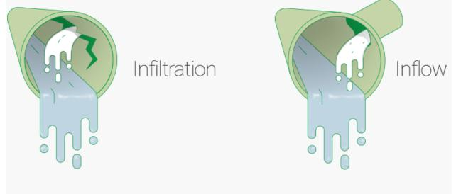
What are examples of Infiltration? Infiltration occurs when groundwater seeps into sewer pipes through cracks, leaky pipe joints and/or deteriorated manholes.
